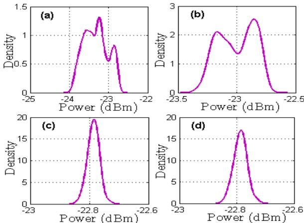
**Fig. 1.** Received power distribution of a selected fog event recorded in Graz on 31.01.2006 for different time durations
