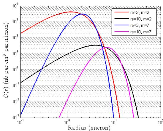
Fig. 3. The MGDSD of fog for different DSD parameter values against  $LWC=0.5 \text{ g/m}^3$ .
