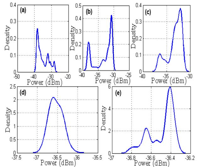
**Fig. 2.** Received power distribution of a selected fog event recorded in Graz on 18-19.11.2009 for different time durations.
