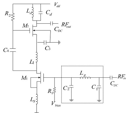
Fig. 1. Complete circuit schematic of the proposed LNA.
