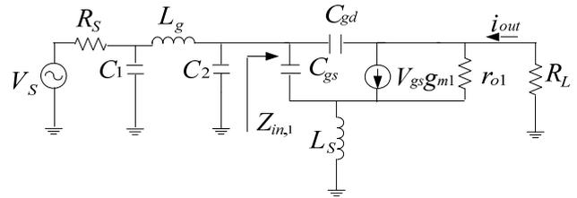
Fig. 4. The small-signal equivalent circuit of  $M_1$ .
