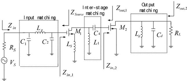
Fig. 3. Circuit schematic of an equivalent two-stage cascaded amplifier.
