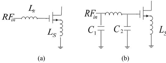
Fig. 2. (a) Conventional input matching topology. (b) The modified input matching topology.
