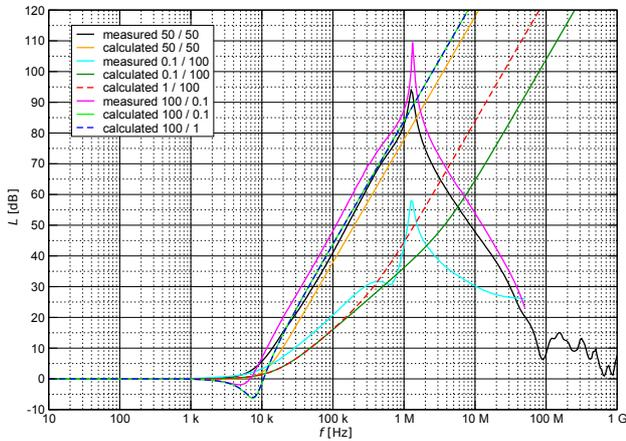
**Fig. 6.** The insertion loss of the Elfis 1ELF16V in asymmetrical systems.
