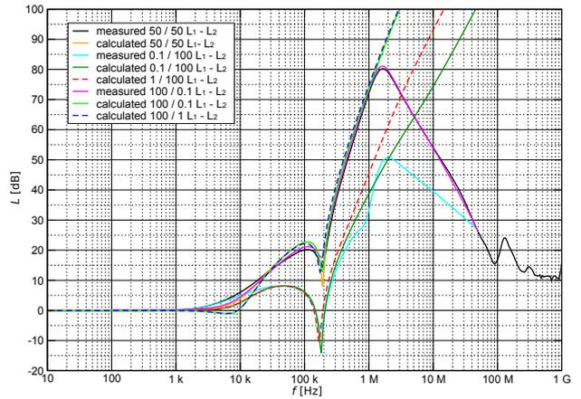
**Fig. 8.** The insertion loss of the Elfis 1ELF16V in "non-symmetrical" systems.
