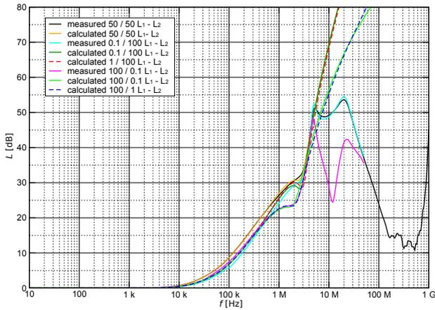
**Fig. 5.** The insertion loss of the Schurter 5110.1033.1 in "non-symmetrical" systems.
