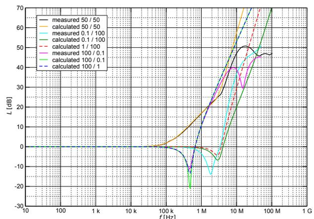
Fig. 4. The insertion loss of the Schurter 5110.1033.1 in symmetrical systems.
