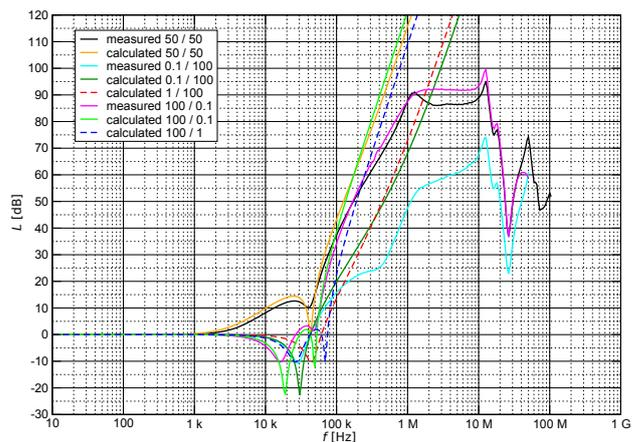
**Fig. 10.** The insertion loss of the Schaffner FN 2070-10-06 in symmetrical systems.
