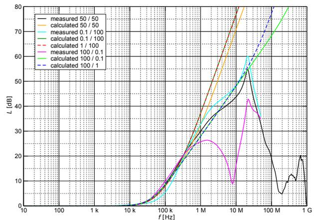
Fig. 3. The insertion loss of the Schurter 5110.1033.1 in asymmetrical systems.
