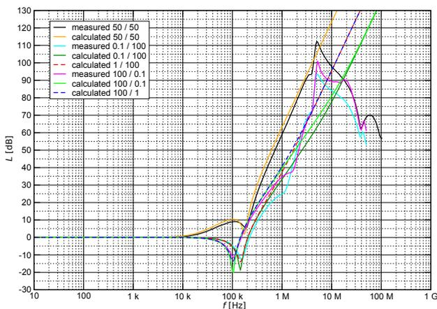
**Fig. 7.** The insertion loss of the Elfis 1ELF16V in symmetrical systems.
