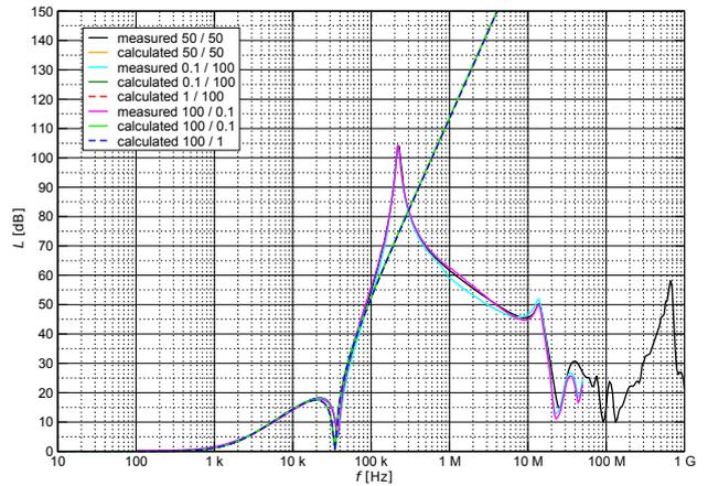
**Fig. 9.** The insertion loss of the Schaffner FN 2070-10-06 in asymmetrical systems.
