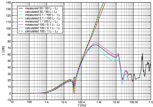
**Fig. 11.** The insertion loss of the Schaffner FN 2070-10-06 in "non-symmetrical" systems.
