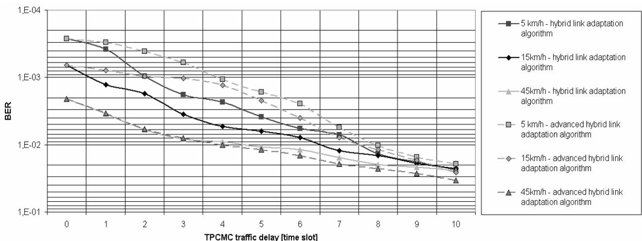
Fig. 4. Average L1 data BERs at various MS velocity and TPCMC traffic delay.
