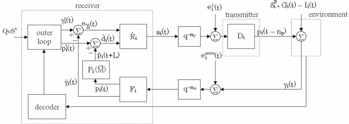
Fig. 1. Principle of basic prediction model.
