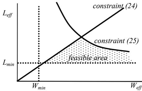
Fig. 9. Design space for switches.
