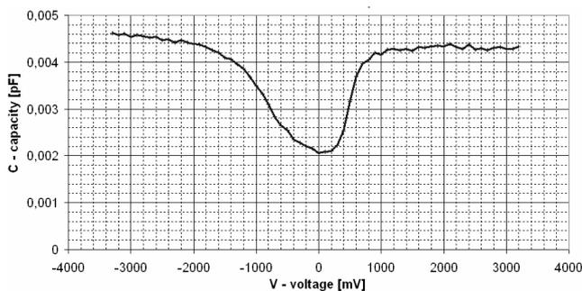
Fig. 13. Nonlinear MOS gate capacitance.
