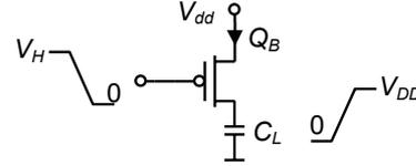
Fig. 8. Equivalent circuit for transient B.
