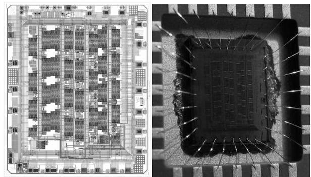
Fig. 12. Top layout and die photograph of test-chip.
