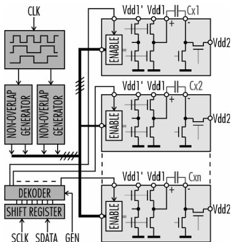
Fig. 10. Block diagram of test-chip.
