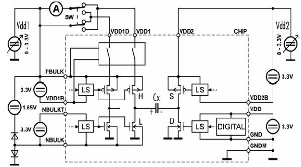
Fig. 11. Schematic diagram of test-chip power supply.
