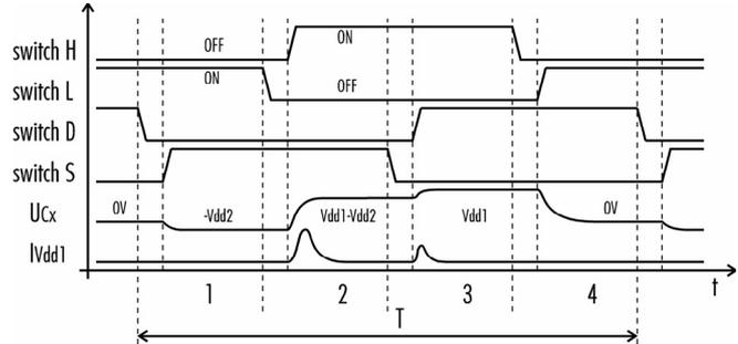
Fig. 3. Waveforms of signals in modified CBCM method.
