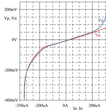
Fig. 8. Measured input characteristics of Current Differencing Unit, transferred to PSpice.
