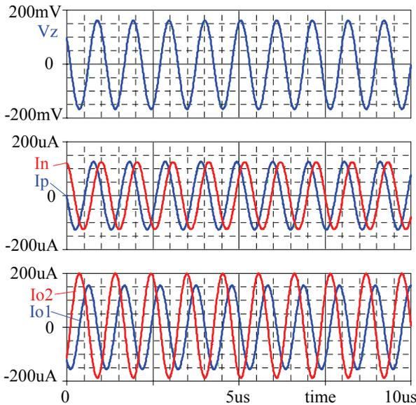
Fig. 9. Simulated steady-state oscillations, CDTA model No. 1,  $f_{osc} = 960 \text{ kHz}$ .
