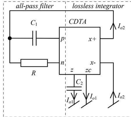
Fig. 3. Proposed CDTA-based quadrature oscillator.
