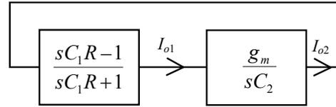
Fig. 2. Block diagram of the quadrature oscillator.
