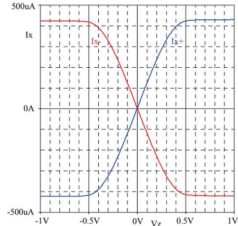
Fig. 7. Measured OTA characteristics, transferred to PSpice.
