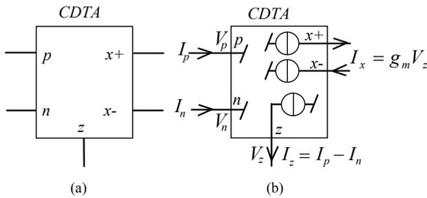
Fig. 1. CDTA (a) schematic symbol, (b) equivalent circuit.
