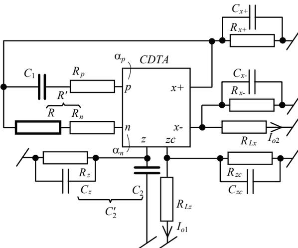
Fig. 6. Modeling linear effects in the oscillator.
