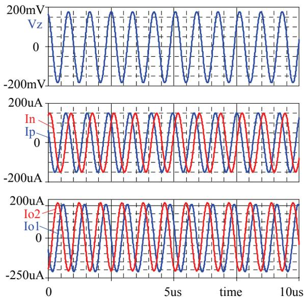
Fig. 11. Simulated steady-state oscillations, CDTA model No. 2, with elimination of real effects,  $f_{osc} = 1.171$  MHz.
