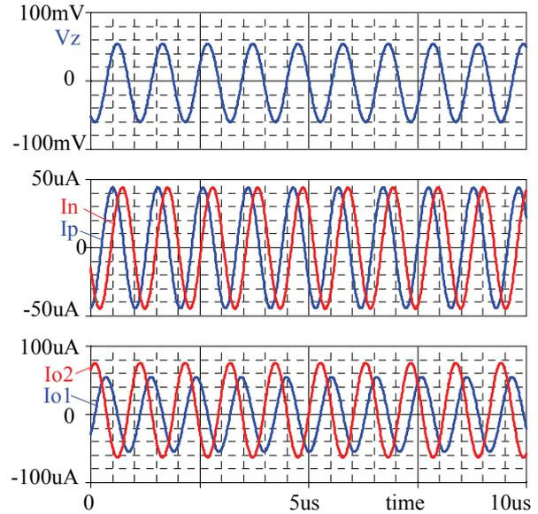
Fig. 10. Simulated steady-state oscillations, CDTA model No. 2,  $f_{osc} = 964 \text{ kHz}$ .
