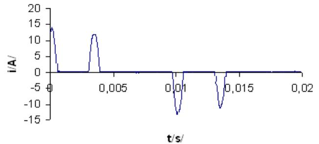
Fig. 3. Input converter current for 4 kW load.
