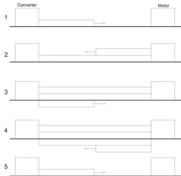
Fig. 5. Reflection of voltage waves between converter and motor.
