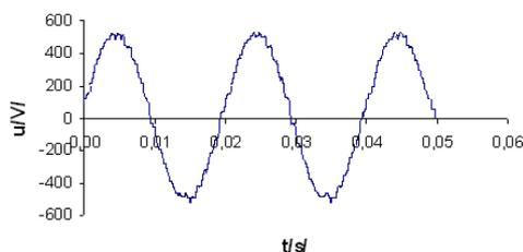
Fig. 6. Sinus filter output voltage.
