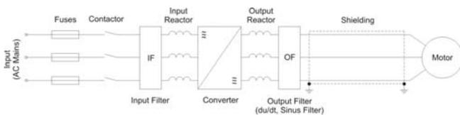
Fig. 2. Frequency converter with typical anti-interference equipment.
