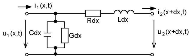
Fig. 4. Cable length element.
