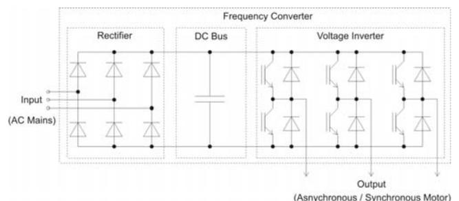
Fig. 1. Topology of frequency converter.
