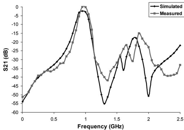
Fig. 7 (a). Transmission co-efficient for 2<sup>nd</sup> iteration.
