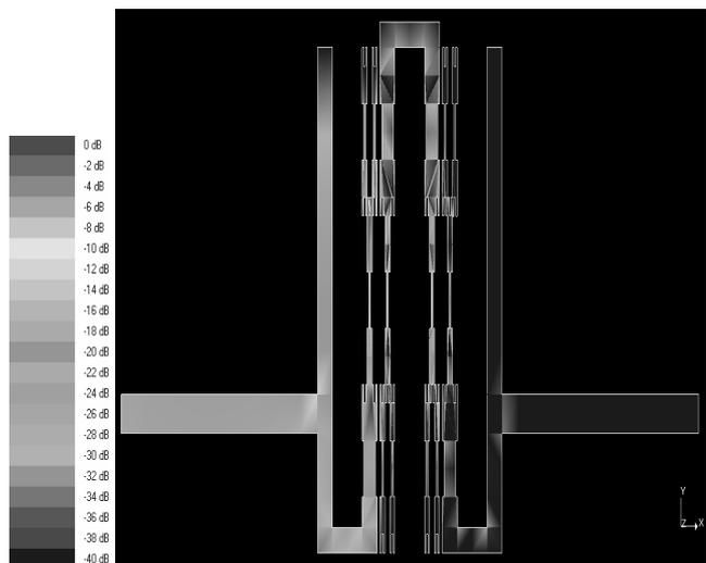
**Fig. 10 (b).** Distribution of the magnitude of the current density on  $f_c = 1$  GHz.
