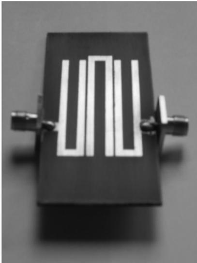
**Fig. 8 (a).** Photograph of hairpin-line filter for zero iteration.
