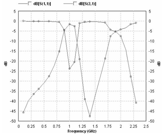
Fig. 2 (b). Frequency response of hairpin-line band pass filter.
