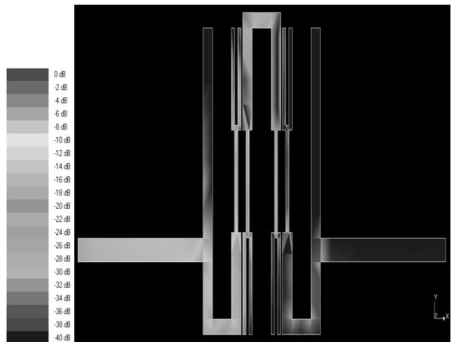
**Fig. 9 (b).** Distribution of the magnitude of the current density on  $f_c = 1$  GHz.
