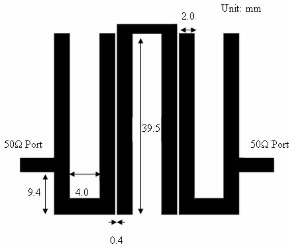
Fig. 2 (a). Layout of hairpin-line band pass filter.
