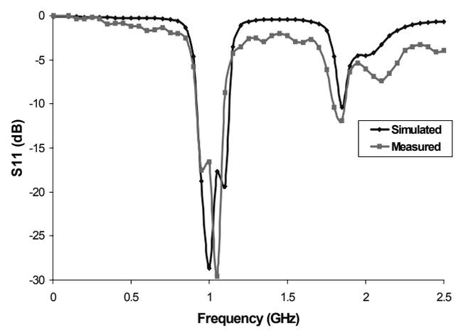
Fig. 5 (b). Reflection co-efficient for zero iteration.
