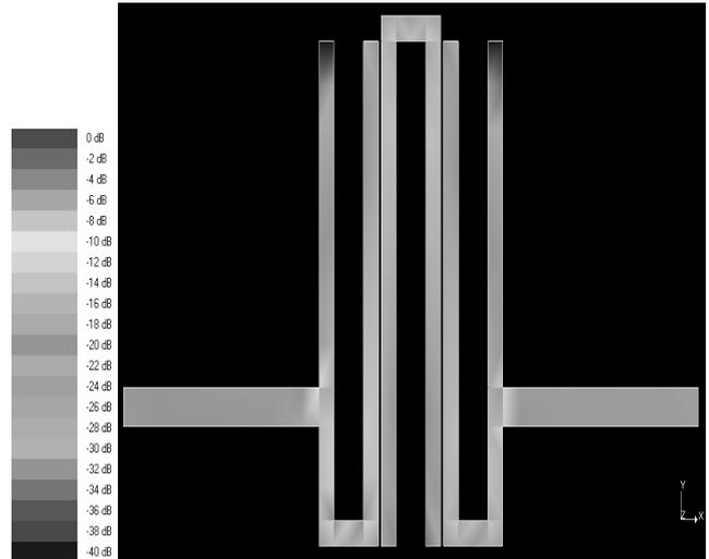
**Fig. 8 (b).** Distribution of the magnitude of the current density on  $f_c = 1$  GHz.
