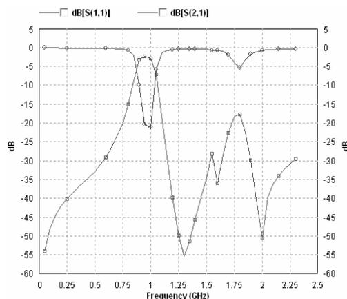
Fig. 4 (b). Frequency response of 2<sup>nd</sup> iteration band pass filter.
