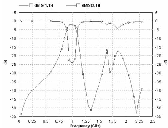
Fig. 3 (b). Frequency response of the 1<sup>st</sup> iteration band pass filter.
