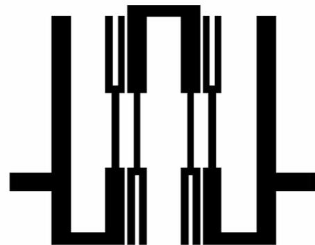
Fig. 3 (a). Layout of the 1<sup>st</sup> iteration fractal band pass filter.
