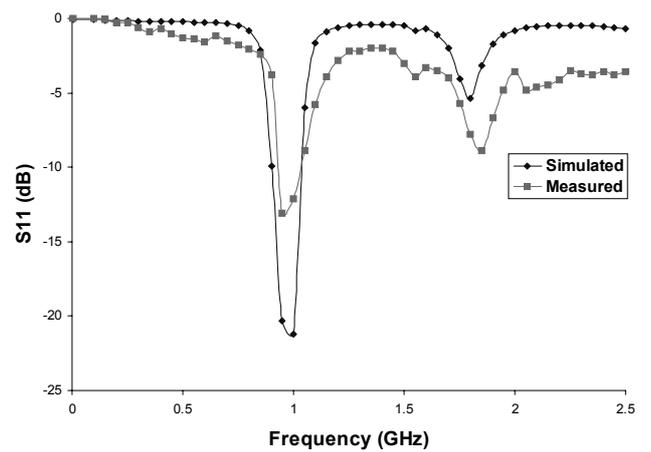
Fig. 7 (b). Reflection co-efficient for 2<sup>nd</sup> iteration.
