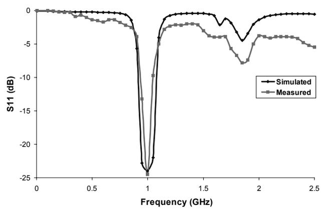
Fig. 6 (b). Reflection co-efficient for 1<sup>st</sup> iteration.
