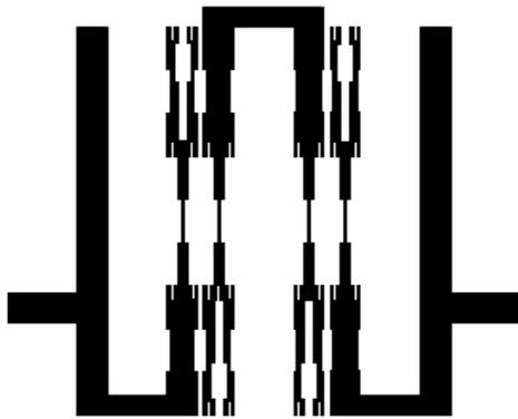
Fig. 4 (a). Layout of the 2<sup>nd</sup> iteration fractal band pass filter.
