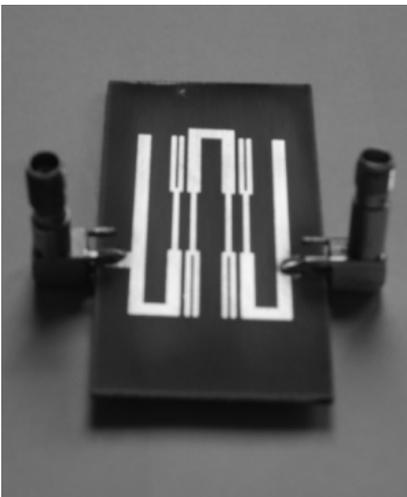
**Fig. 9 (a).** Photograph of hairpin-line filter for 1<sup>st</sup> iteration.
