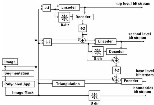
Fig. 1. Block diagram of the three-level hierarchical encoder.
