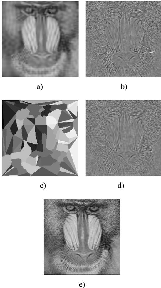
**Fig. 5.** Base level processing: a) the upsampled decoded image from second level (Fig. 4f) using B-spline interpolation, b) the difference between the original (Fig. 2a) and a), c) the image mask for base level – triangulated Fig. 2b), d) the decoded difference b) (0.35 bpp), e) sum of a) and d) - final product of the decoding process (0.5 bpp; PSNR 23.22 dB).
