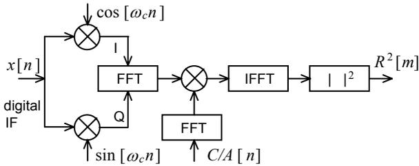
Fig. 4. Non coherent Correlator in frequency domain.
