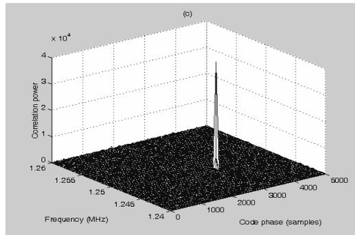
**Fig. 7.** Correlation matrix for satellite 19 with  $N(10, 0.1)$ . (a) with FFT search (5000 points), (b) with signal decimation (from 5000 to 2500 points) and (c) with lifting wavelet decomposition (from 5000 to 1250 points).
