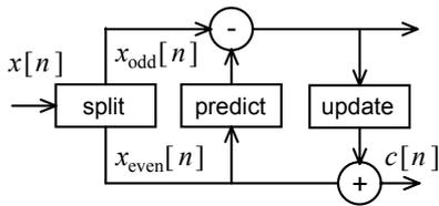
Fig. 1. The lifting scheme, forward transform: Split, Predict and Update phases.
