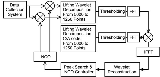
Fig. 5. Acquisition using lifting wavelet decomposition.
