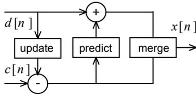
Fig. 2. The lifting scheme, inverse transform: Update, Predict and Merge stages.
