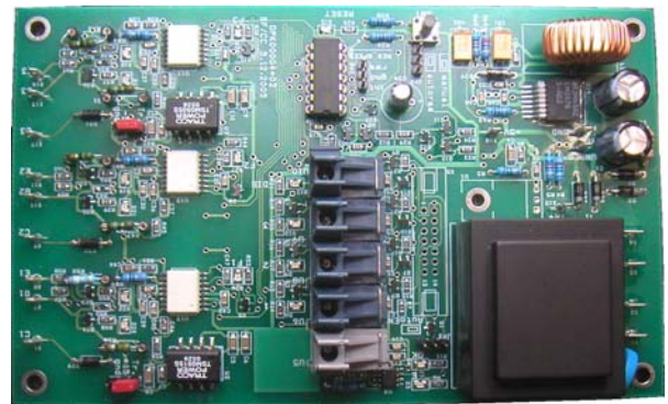
Fig. 8. The driver unit for three transistors at the same collector voltage potential.
