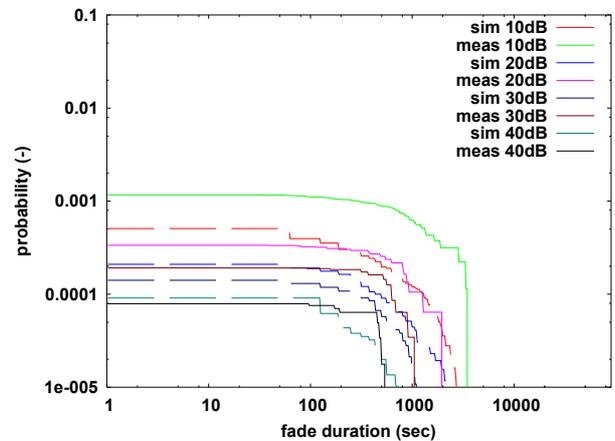
Fig. 9. Fade duration statistics obtained from measured and simulated time series for path TESCO - Chloumek, year 2003.
