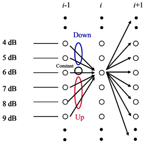
Fig. 2. DLR channel model as a discrete-valued 2<sup>nd</sup> order Markov chain. Grouping of transitions allows for a reduction of the number of transition probabilities.
