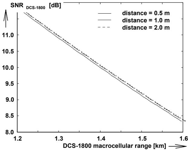
Fig. 2. DCS-1800 SNR as a function of DCS-1800 macrocellular range for 3 different distances between the UWB transmitter and DCS-1800 receiver when  $P_{UWB} = -90$  dBm/MHz.
