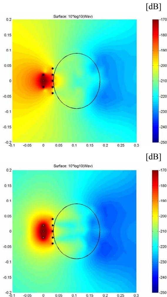
**Fig. 6.** Graphical plots showing the power density inside the human head phantom before (top figure) and after (bottom figure) the Least Mean Square solution is applied, which respectively corresponds to plots b and e in Fig. 5.
