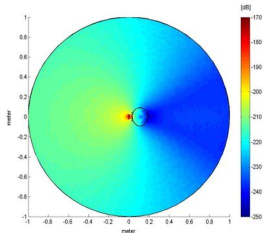
Fig. 3. A surface plot showing the calculated magnitude of the power density based on the electric field solution.
