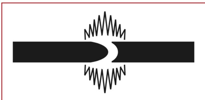
Fig. 1. Classical diagram of a DC electric arc. During the operation the positive electrode was used up much faster, thus forming a crater on its tip.
