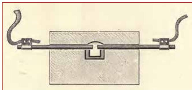
FIG. 6. Diagram of the electric arc furnace as described by Moissan (from Ref. 5).
