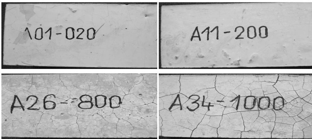
Fig. 4. The photo of selected specimens after the three-point bending test.
