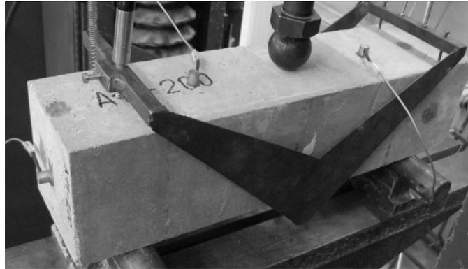
Fig. 1. The arrangement of acoustic emission sensors on specimen during the three-point bending test.
