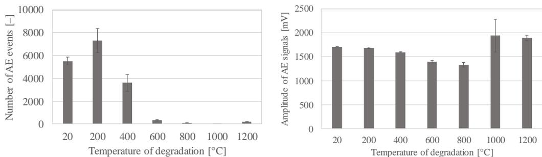
Fig. 3. The dependence of number of AE events (left) and amplitude of AE signals (right) on thermal stress level (record a whole of measurement).
