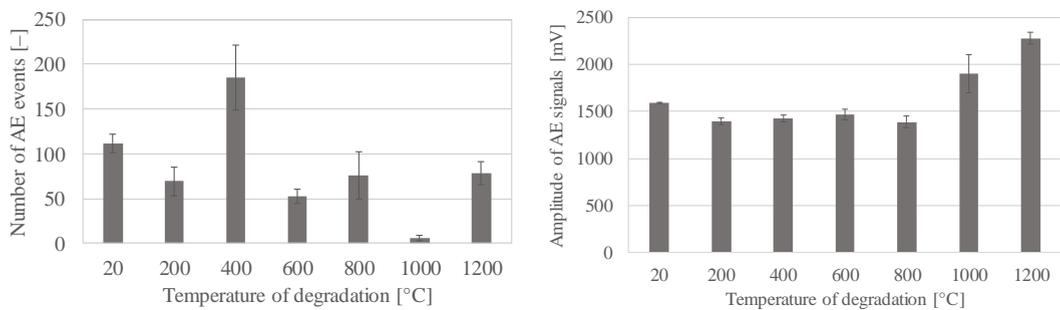
Fig. 2. The dependence of number of AE events (left) and amplitude of AE signals (right) on thermal stress level (record to ultimate tensile capacity).
