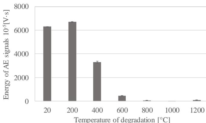
Fig. 5. The dependence of energy of AE signals on degradation thermal stress level (record a whole of measurement).
