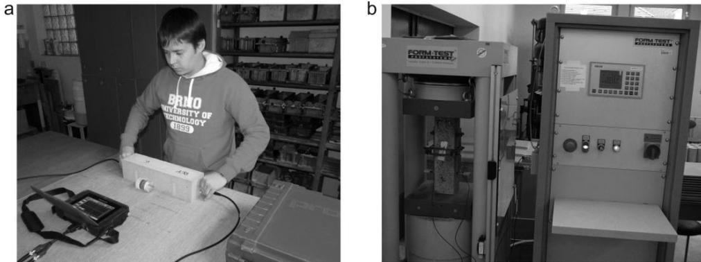
Fig. 1. (a) Determination of the dynamic modulus of elasticity  $E_{cu}$  using the ultrasonic pulse velocity test; (b) determination of the static modulus of elasticity  $E_c$ .
