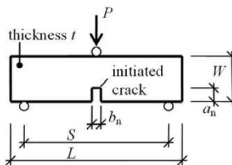
Fig. 1. Schematic of three-point bend (3PB) specimen geometry
