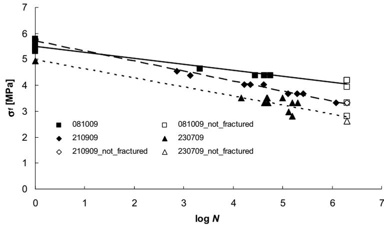
Fig. 2.  $\sigma_f$ - $N$  diagrams for 230709, 210909 and 081009 materials (full symbol: broken specimen; empty symbol: unbroken specimen)
