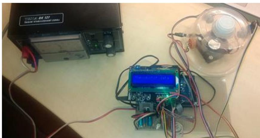
**Figure 1** Experimental prototype of the electronic nose.
