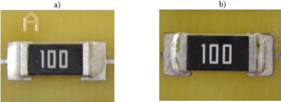
**Figure 2:** Solder joints soldered by different methods – a) Solder joints with solder preforms in the flux b) Solder joints with solder paste printed through the stencil
