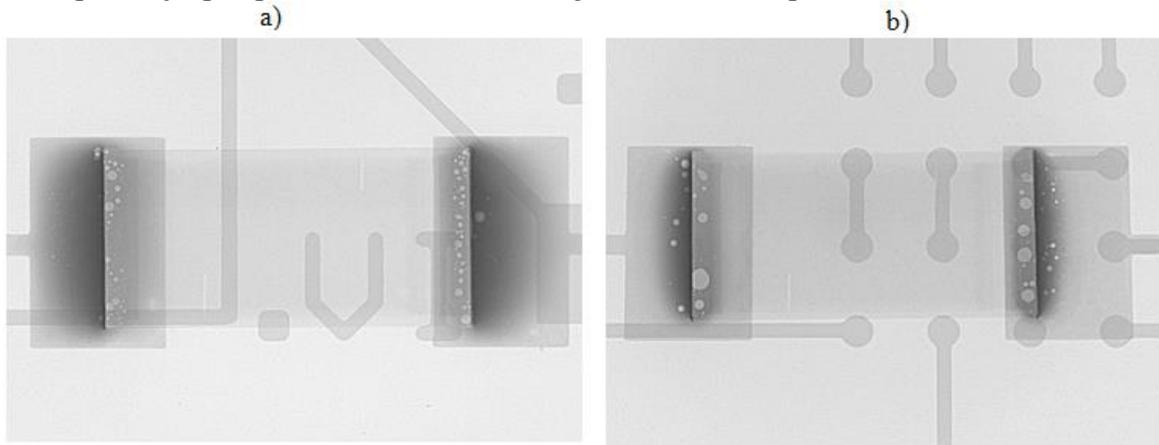
**Figure 3:** X-ray analysis of solder joints soldered by different methods – a) Solder joints with solder preforms in the flux b) Solder joints with solder paste printed through the stencil
