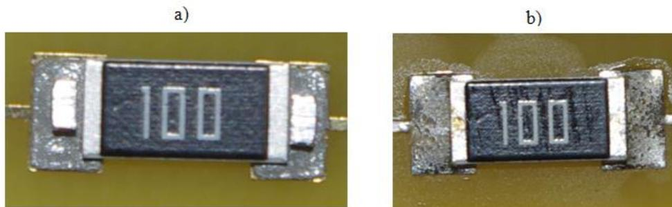
**Figure 4:** Solder fortification method – (a) Solder preforms mounted to paste before soldering in vapors (b) Solder preforms and solder paste after soldering in vapors
