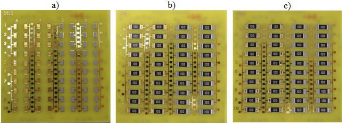
**Figure 1:** Process of manufactory of solder joint with solder preforms: a) Printed flux and solder paste through the stencil b) Mounted SMD 2512 components to flux and solder paste c) Added solder preforms to flux and SMD 2512 components [4]
