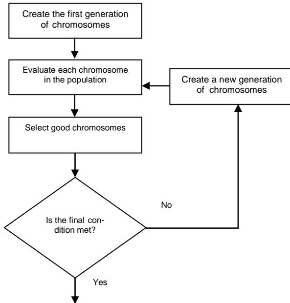
**Fig. 1: Diagram of a genetic algorithm**
