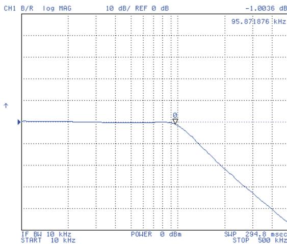
Fig. 8. Measured frequency response of the wave active filter.
