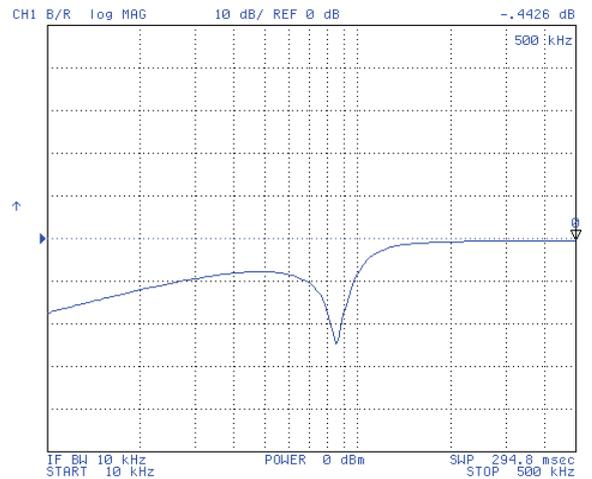
Fig. 9. Measured power complementary frequency response of the wave active filter.
