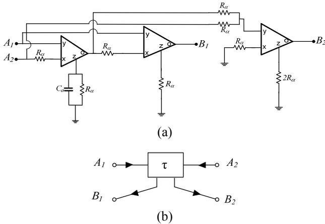
Fig. 5. CFOA based wave equivalent of an inductor in series-branch: (a) Circuit level representation, (b) the used symbol.
