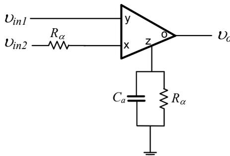
Fig. 2. CFOA based lossy integration-subtraction block.
