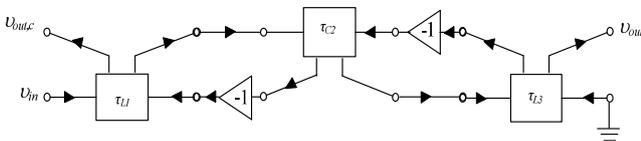
Fig. 7. Block diagram of the corresponding wave active filter.
