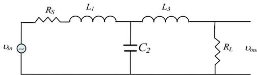
Fig. 6. 3<sup>rd</sup>-order LC ladder prototype filter.
