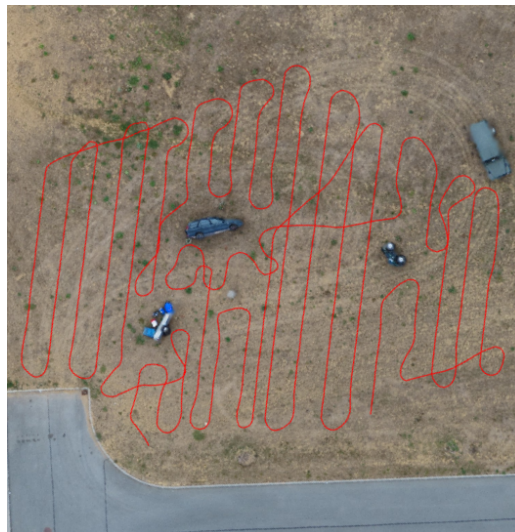
Fig. 5.1: The picture shows the terrestrial radiation mapping with a planned trajectory in a real-world experiment
