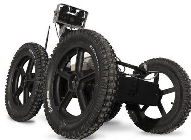
Fig. 3.1: Four-wheel Orpheus X4 robot for work in inaccessible or dangerous areas ( http://cafr.cz/orpheus---x4.html )
