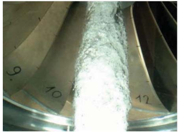
Figure 2: Straight cavitating vortex rope (full load operation) [3]
