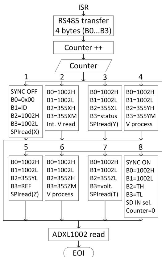
Figure 4. Flowchart of the interrupt service routine.
