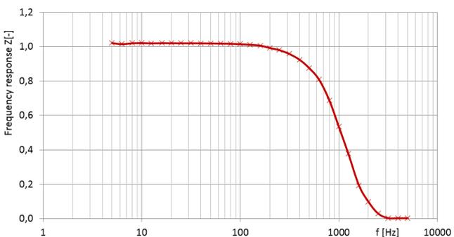
Figure 9. Frequency response of ADXL355 sensor (Z axis).
