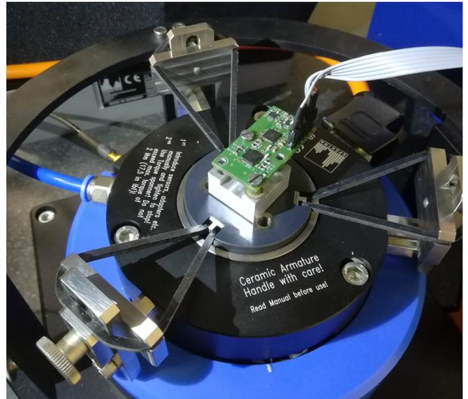
Figure 5. Photo of the SVS during tests on SPEKTRA system (measurement in Z axis is shown).
