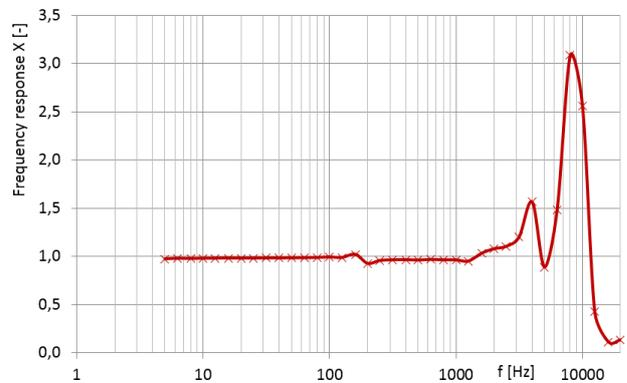
Figure 6. Frequency response of ADXL1002 sensor.
