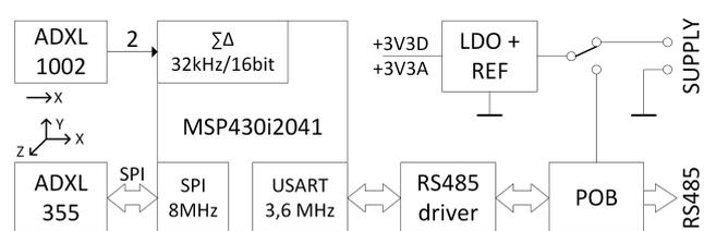
Figure 1. Block schematics of the Smart Vibration Sensor
