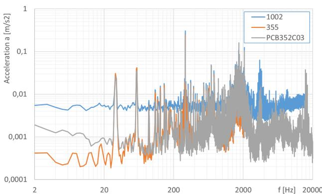
Figure 12. Acceleration spectrum for all three sensing elements.
