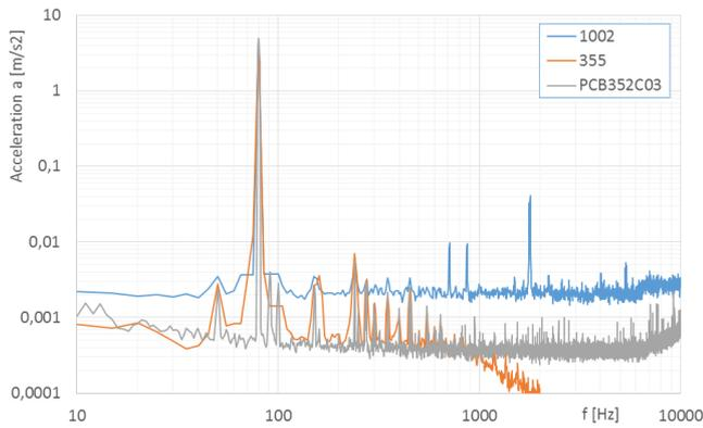
Figure 14. Acceleration spectrum measured on vibration exciter driven with 80 Hz sine wave.
