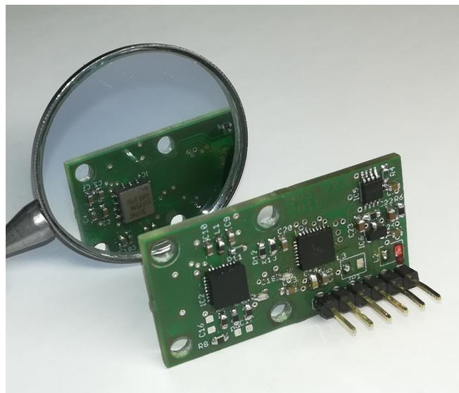
Figure 2. Photography of the Smart Vibration Sensor PCB.
