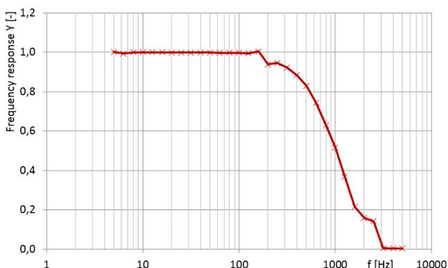
Figure 8. Frequency response of ADXL355 sensor (Y axis).
