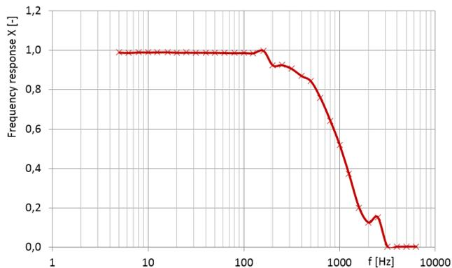
Figure 7. Frequency response of ADXL355 sensor (X axis).
