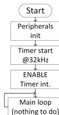
Figure 3. Flowchart of embedded software of Smart Vibration Sensor.
