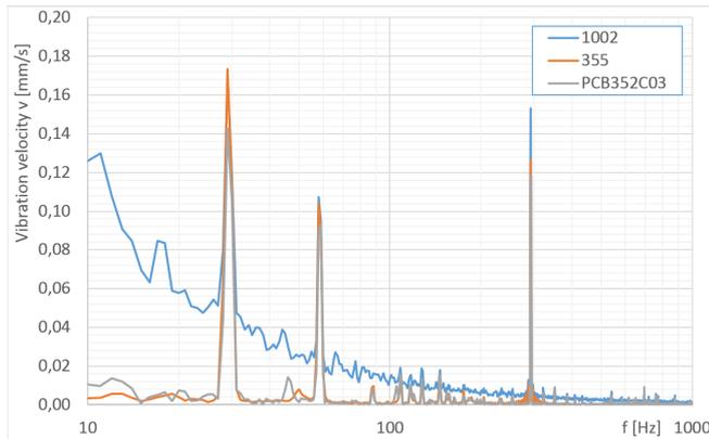
Figure 11. Vibration velocity of the stepper motor measured by the SVS and compared with output data measured by a standard accelerometer.
