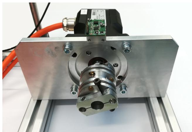
Figure 10. Stepper motor with bellows clutch and SVS.
