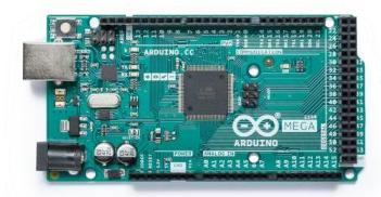
Figure 4.2: Original Arduino Mega 2560 board [13].
