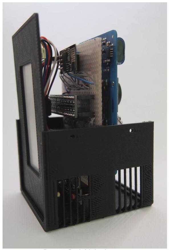
Figure 4.22: Detail of the board mounting.
