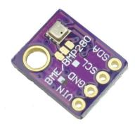
Figure 4.5: A BME280 sensor on a breakout board [8].
