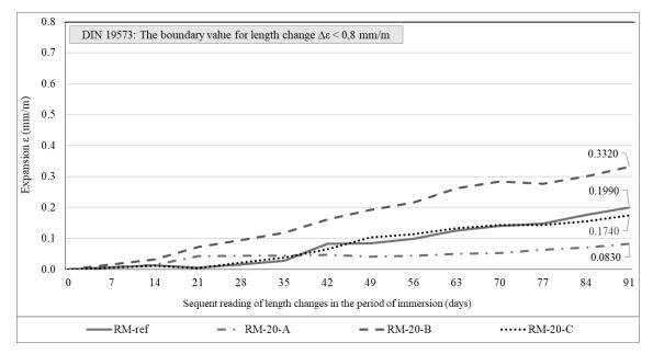
Figure 1. Graphical representation of the course of deformation of test specimens exposed to sulphates in time.
