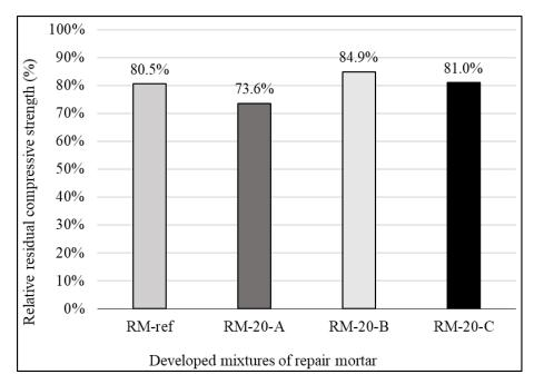
**Figure 2.** Graphical representation of the relative residual compressive strength of the corroded mortar test samples after exposed to a chemically aggressive solution of sulfuric acid ( $H_2SO_4$ ) with a concentration of pH = 0 (c( $H_2SO_4$ ) = 1.0mol / 1) for 14 days.
