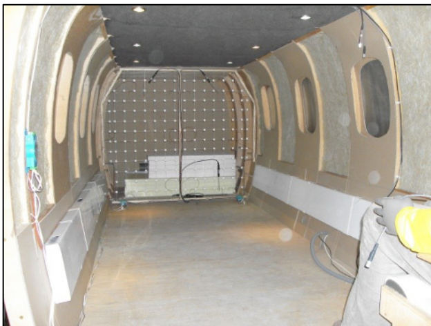
Fig. 3. Real interior of small aircraft cabin mock-up (main door to cockpit view).
