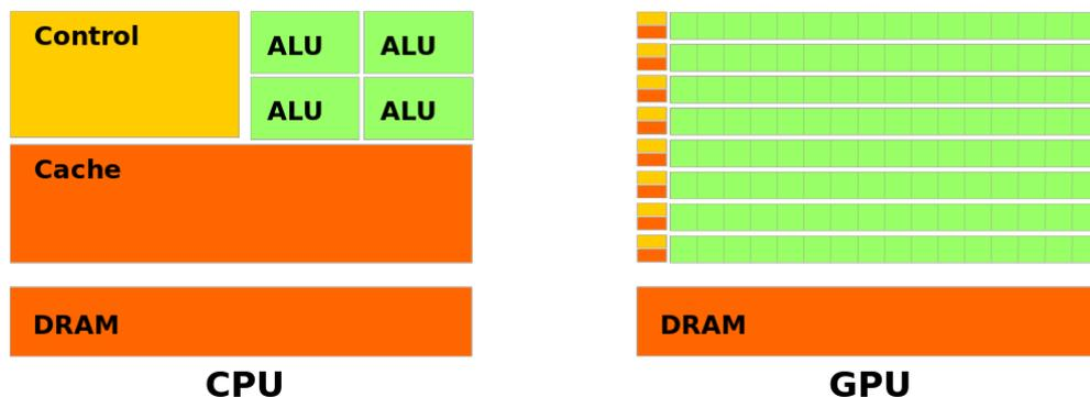
Figure 1.1: CPU and GPU architecture comparison (taken from [15])
