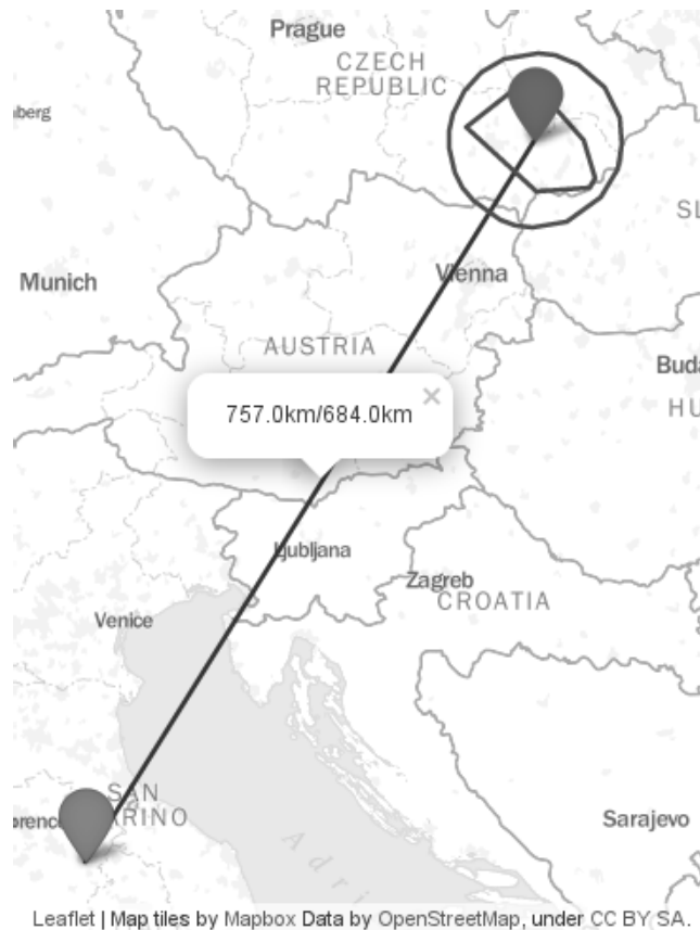
FIGURE 10. Example results for www.slunecnireality.cz – web-content projected area (polygon), extended web-content projected area (circle), found location of hosted web server, and distances to web server from area centroid and border of extended projected area.
