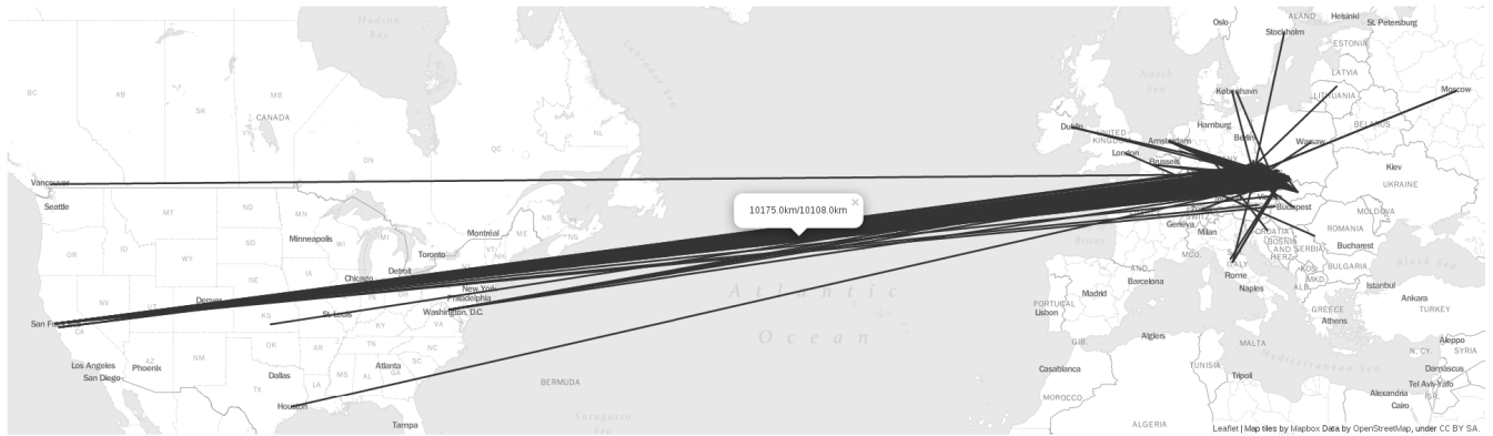
FIGURE 13. Global picture of web server location with large over-distances from their content-projected area.
