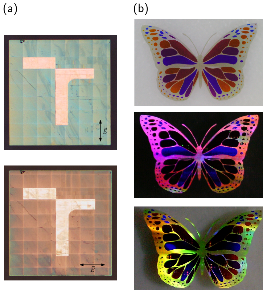
Figure 5.10 (a) prototype of OVD made of silver rectangular antennas illuminated by two different polarizations, (b) prototype of OVD made of aluminum nanodiscs illuminated under different angles, adapted from [129]
