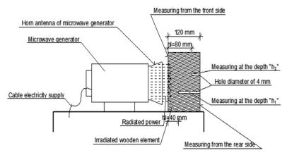
Fig. 2. View of diagram of wood element during irradiation
