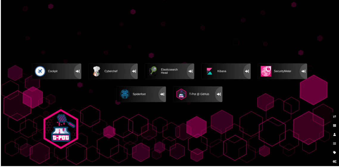
Fig. 3.2: T-pot web dashboard and application launcher, displaying all available tools.
