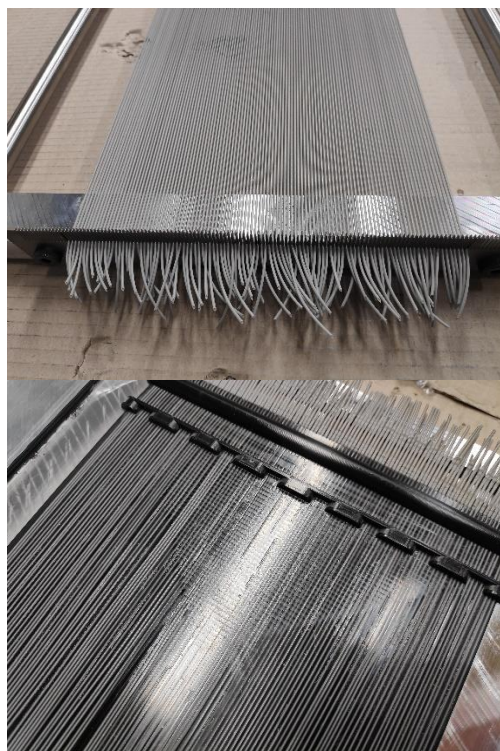
Fig. 6. Parallel fibers before the RIM process at the top and the final planar heat exchanger at the bottom.
