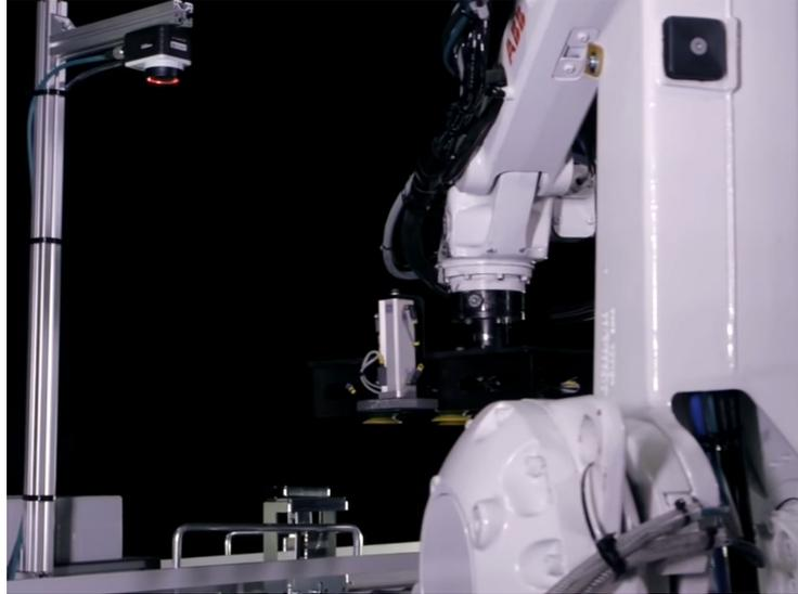
Figure 3.17: ABB vision system for robot guidance [22]
