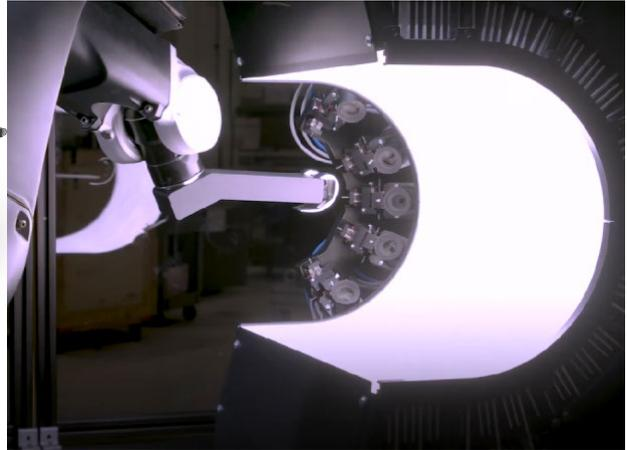
Figure 3.4: Zeiss Surfmax optical system [11]
