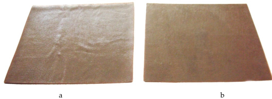
Figure 7. Glass-fibre reinforced plastic specimens obtained by moulding modes No 1 (a) and No 2 (b).
