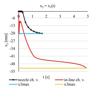
**Fig. 11.** 1AM in-line valve and nozzle check valve simulations in the piping system in case of a sudden failure of centrifugal pump during a power outage, the disc and the poppet positons.
