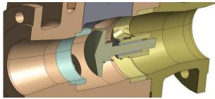
Fig. 2. In-line check valve.
