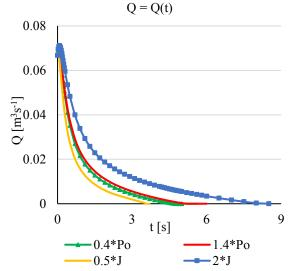
Fig. 13. 1DOF CFD and 1AM simulations of the in-line check valve, the flow rate.
