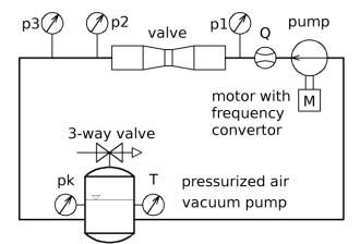
Fig. 3. The pipeline and the testing circuit diagram
