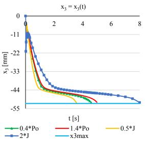
Fig. 14. 1DOF CFD and 1AM simulations of the in-line check valve, the positions of the poppet.
