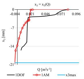
**Fig. 7.** 1DOF CFD and 1AM simulations of the disc position of the nozzle check valve, Ts = 1.5s.
