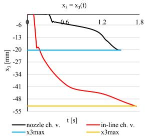
**Fig. 9.** 1AM simulations of the in-line and nozzle check valve in the piping system, the disc and the poppet positons.
