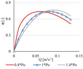
Fig. 12. The pump efficiency curves.
