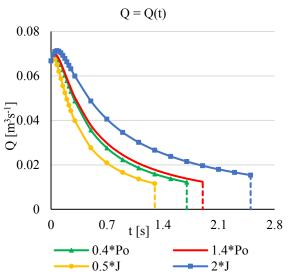
Fig. 15. 1DOF CFD and 1AM simulations of the nozzle check valve, the flow rate.
