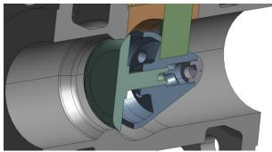
Fig. 1. Nozzle check valve.
