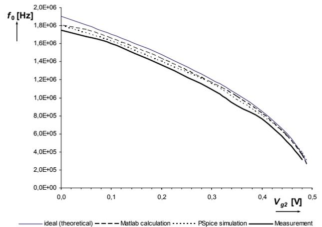
Fig. 10. Oscillation frequency versus control voltage.
