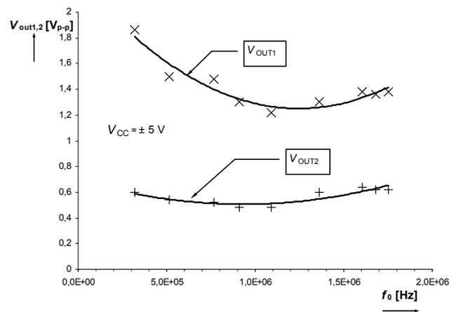
Fig. 11. Output voltages vs. oscillation frequency (measured).
