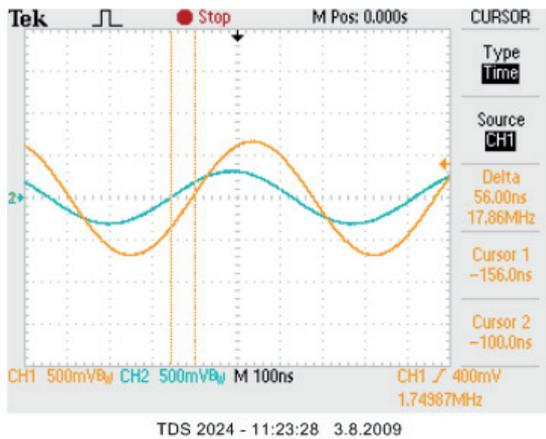
Fig. 8. Measured output signals (larger is  $V_{OUT1}$ , smaller is  $V_{OUT2}$  for  $V_{g1} = 2 \text{ V}$ ,  $V_{g2} = 0 \text{ V}$ )
