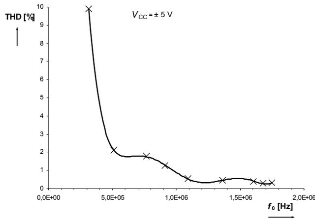
Fig. 12. THD versus oscillation frequency (measured).
