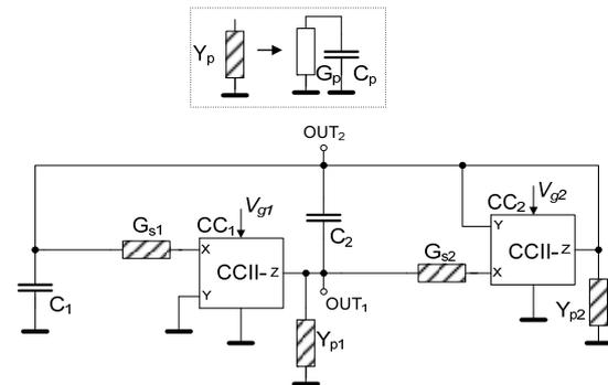
Fig. 14. Important parasitic influences in the proposed oscillator.
