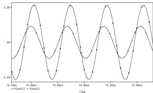
**Fig. 6.** Time waveforms of the output signals (for  $V_{g1} = 2$  V,  $V_{g2} = 0$  V), given by simulation (transient analysis in PSpice).
