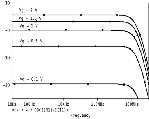
Fig. 2. Magnitude response as a function of driving voltage  $B = B(f, V_g)$ .
