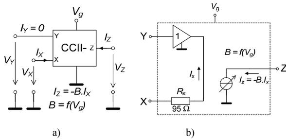
Fig. 1. Principle of adjustable CCII-: a) Symbol, b) model.
