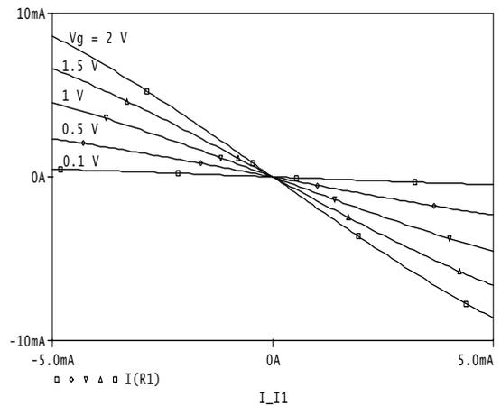
Fig. 3. Input-output current characteristics  $I_z = f(I_x, V_g)$ .
