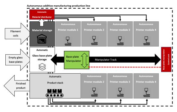
Figure 1: Topology of autonomous additive manufacturing production line.
