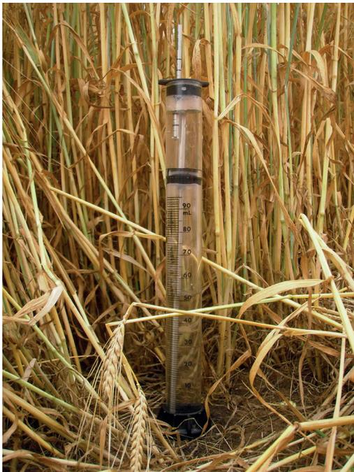
2: Mini Disc Infiltrometer
