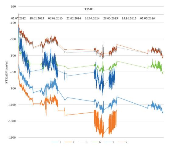
Fig. 4. Long-term monitoring of deformation  $[\mu m/m]$ . In the middle section is strain highest (gauges no. 1 and 2)
