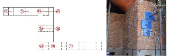
Fig. 2. (a) Plan of vertical prestressing; (b) View of measured model (three brick walls)
