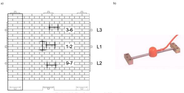
Fig. 3. (a) Labelling of strain gauges; (b) Wire strain gauges
