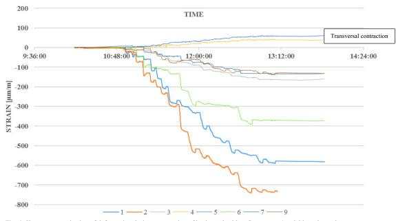
Fig. 6. Short-term monitoring of deformation during prestressing of horizontal cables. Gauges no. 4 and 5 have been shown transverse contraction
