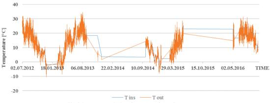
Fig. 5. Long-term monitoring of masonry surface and core temperature.
