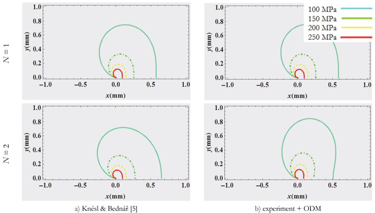
Figure 3:  $\sigma_{\text{IMH}}$  crack tip stress approximation considering one and two initial terms of the Williams expansion on specimen denoted as YX9\_a6\_im16 ( $P = 3.706 \text{ kN}$ ,  $a = 22 \text{ mm}$ ): a) stress values calculated from the coefficients determined theoretically [5]; b) stress values calculated from the coefficients obtained by means of the ODM from the experimental measurements.
