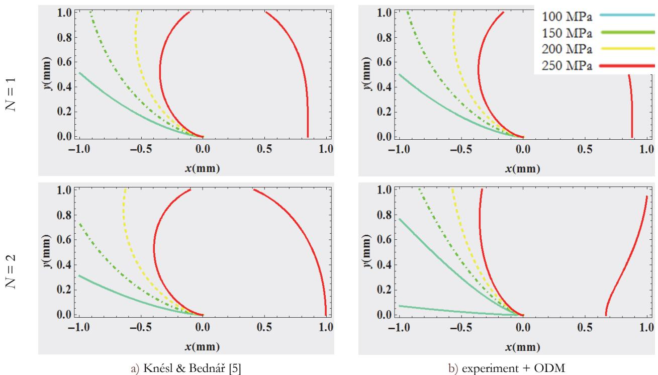
Figure 5:  $\sigma_{\text{HMH}}$  crack tip stress approximation considering one and two initial terms of the Williams expansion on specimen denoted as YX9 a19\_im30 ( $P = 7.060$  kN,  $a = 28.62$  mm): a) stress values calculated from the coefficients determined theoretically [5]; b) stress values calculated from the coefficients obtained by means of the ODM from the experimental measurements.
