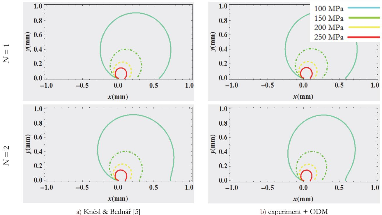
Figure 2:  $\sigma_1$  crack tip stress approximation considering one and two initial terms of the Williams expansion on specimen denoted as YX9 a6\_im16 ( $P = 3.706 \text{ kN}$ ,  $a = 22 \text{ mm}$ ): a) stress values calculated from the coefficients determined theoretically [5]; b) stress values calculated from the coefficients obtained by means of the ODM from the experimental measurements.
