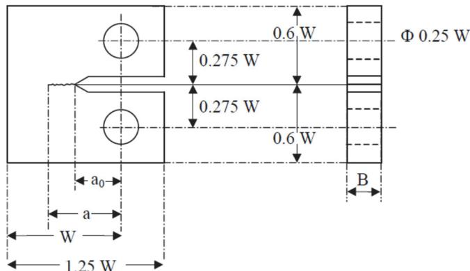
Figure 1: Geometry of the compact tension (CT) specimen in accordance with ASTM standard [6].  $W=48$  mm,  $B=24$  mm.
