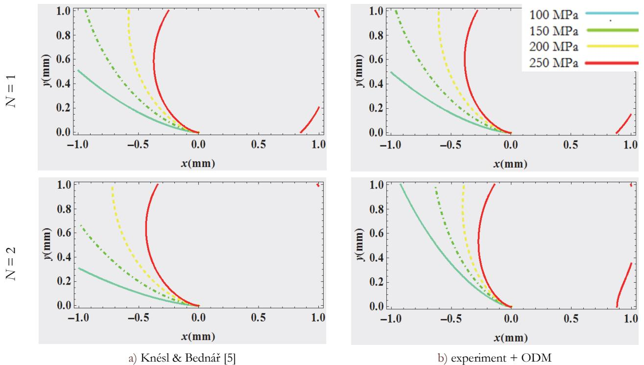
Figure 4:  $\sigma_1$  crack tip stress approximation considering one and two initial terms of the Williams expansion on specimen denoted as YX9\_a19\_im30 ( $P = 7.060 \text{ kN}$ ,  $a = 28.62 \text{ mm}$ ): a) stress values calculated from the coefficients determined theoretically [5]; b) stress values calculated from the coefficients obtained by means of the ODM from the experimental measurements.
