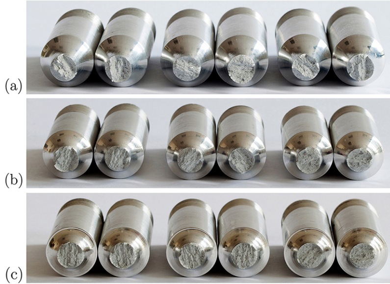
Figure 5.21: Post-mortem notched cylindrical specimens: (a) with d_0 = 9 mm, R = 13 mm; (b) with d_0 = 9 mm, R = 6.5 mm; (c) with d_0 = 9 mm, R = 4 mm.
