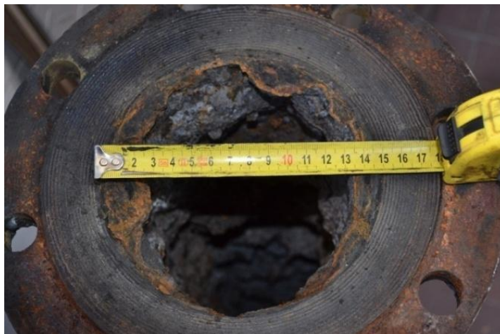
Picture 4.9. – Clogging of cast iron pipe by carbonic accretions at SLKP, a. s.
