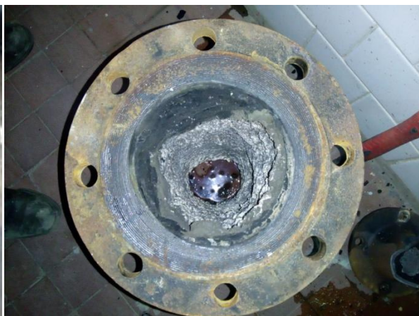
Picture 2.5. – Damaged cast iron pipeline after few years by incrust
