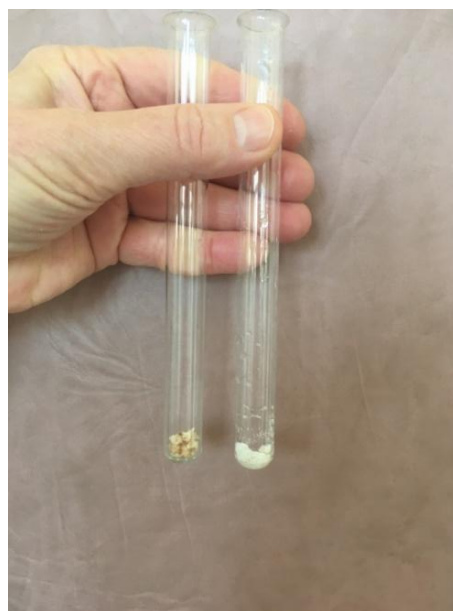
Picture 4.15. – Incrust sample on the left side, indissoluble silicate on the right side
