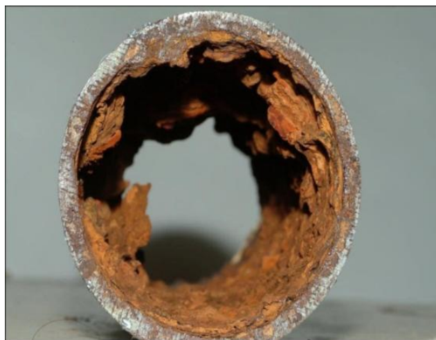
Picture 2.7. – Corrosion in pipeline [6]
