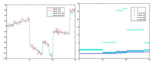
Figure 4: Approximating randomly generated signal after second step  $\lambda_a = 8$  and  $\lambda_b = 0.15$ . SNR of the observed signal is SNR = 18.91dB, of the recovered signal after second step  $SNR_{FB} = 31.03dB$ ,  $SNR_{DR} = 31.03dB$ .
