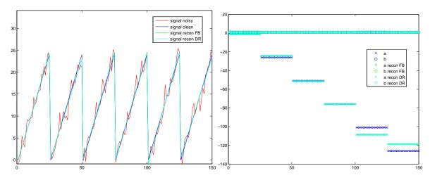
**Figure 2:** Approximating sawtooth signal after second step with  $\lambda_a = 0.075$  and  $\lambda_b = 0.075$ . SNR is SNR = 19.68dB, of the recovered signal after second step  $SNR_{FB} = 30.77dB$ ,  $SNR_{DR} = 30.77dB$ .
