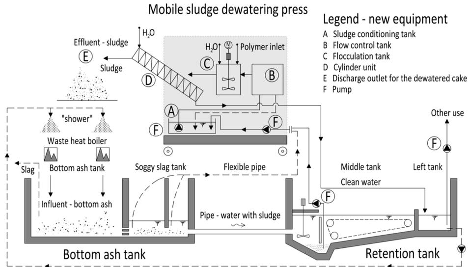
Figure 2. Process diagram of optimized SM.
