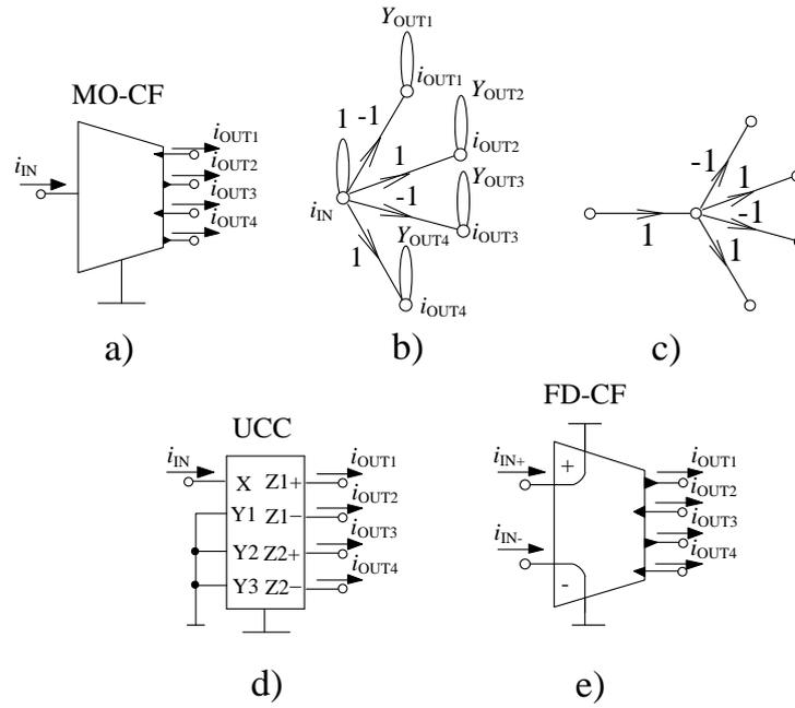
**Figure 5.1** a) schematic symbol of the MO-CF, b) modified M-C graph of the MO-CF, c) simplified M-C graph of the MO-CF, d) possible implementation of the MO-CF using the UCC, e) schematic symbol of the FD-CF
