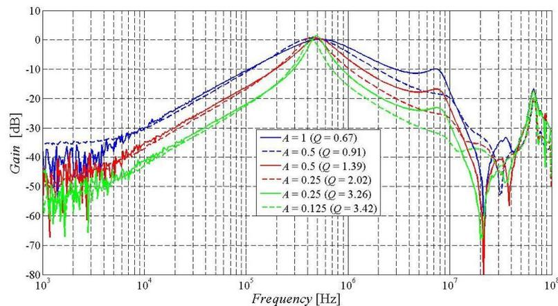
**Figure 6.5 Comparison of possibility to adjust the quality factor when comparing experimental results: S-E filter from Fig. 6.1 (solid lines), F-D filter from Fig. 6.2 (dashed lines)**
