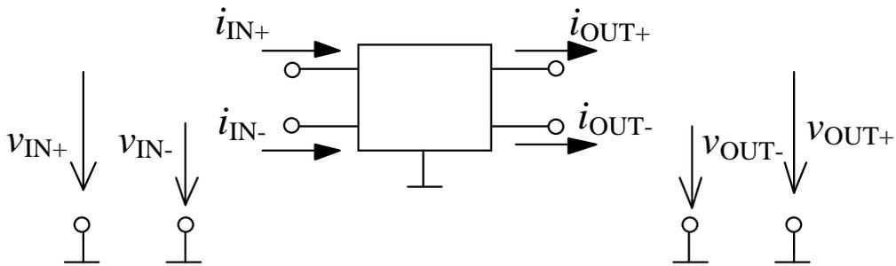
Figure 3.2 Structure used to illustrate the fully-differential general current transfer
