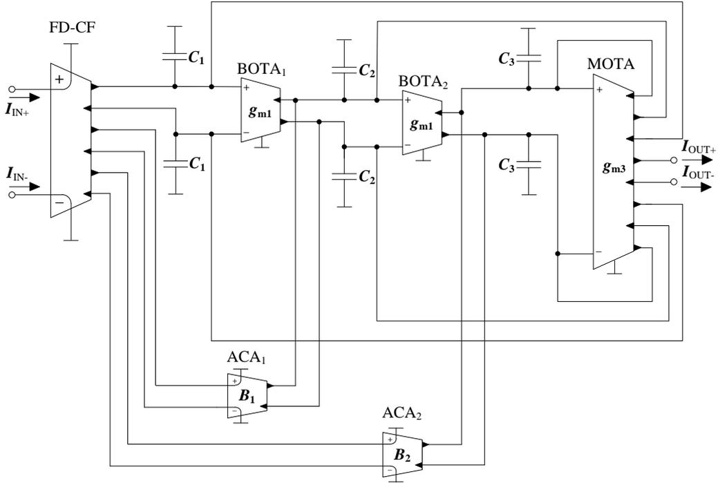
**Figure 7.3 Fully-differential form of the proposed  $(1 + \alpha)$ -order low-pass filter**
