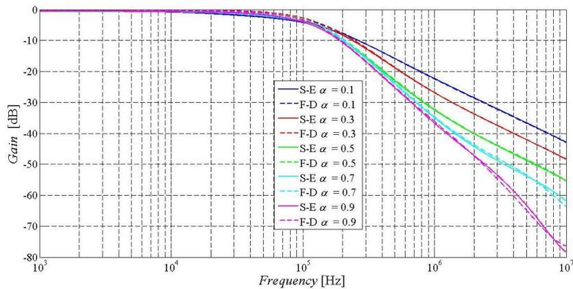
**Figure 7.4** Comparison of simulated transfer functions of the S-E filter from Fig. 7.2 (solid lines) and the F-D filter from Fig. 7.3 (dashed lines) when  $\alpha$  was set to 0.1, 0.3, 0.5, 0.7 and 0.9
