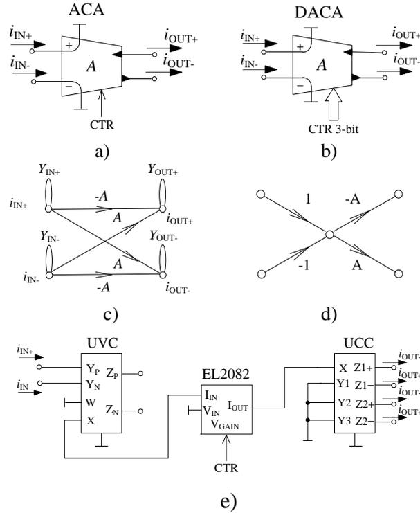
**Figure 5.3** a) schematic symbol of the ACA, b) schematic symbol of the DACA, c) modified M-C graph of the DACA, d) simplified M-C graph of the DACA, e) alternative implementation of the DACA using one UCC, UVC and EL2082
