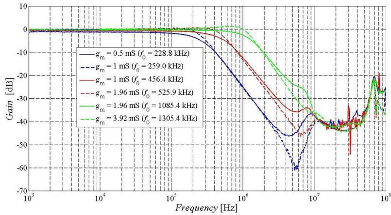
**Figure 6.4 Comparison of possibility to control the pole frequency when comparing experimental results: S-E filter from Fig. 6.1 (solid lines), F-D filter from Fig. 6.2 (dashed lines)**
