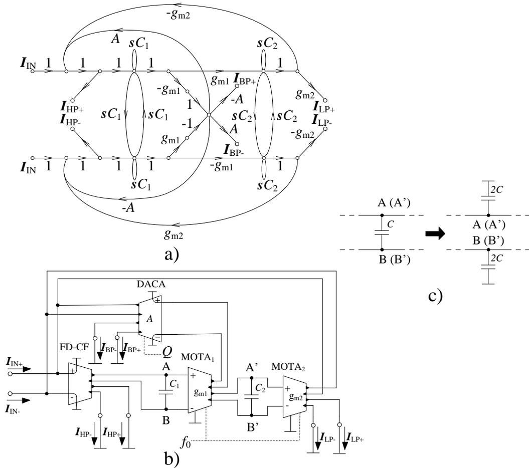
**Figure 6.2 Fully-differential form of the filter with two OTAs, one DACA and one CF:**
