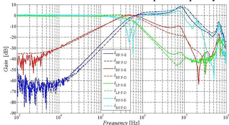
**Figure 6.3 Comparison of transfer functions high-pass, band-pass, low-pass and band-stop of experimental results: the S-E filter from Fig. 6.1 (solid lines) and the F-D filter from Fig. 6.2 (dashed lines)**
