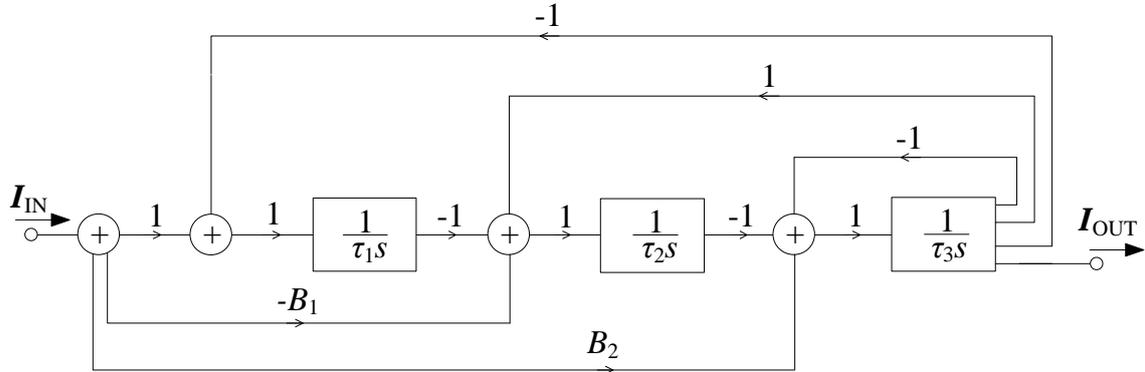
**Figure 7.1** Block diagram of the third-order IFLF topology filter leading to  $(1 + \alpha)$ -order low-pass filter
