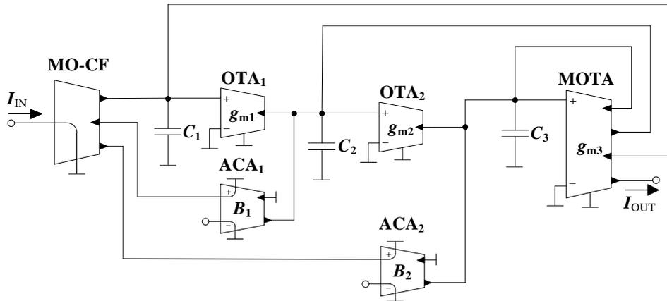
**Figure 7.2** Single-ended form of the proposed S-E  $(1 + \alpha)$ -order low-pass filter
