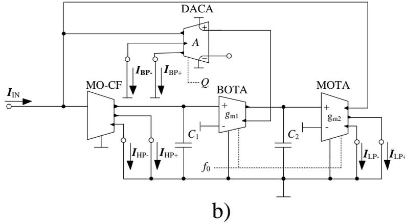
**Figure 6.1** Single-ended form of the filter with two OTAs, one DACA and one MO-CF:
