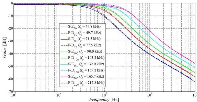
Figure 7.5 Comparison of ability to control the pole frequency of the S-E filter from Fig. 7.2 (solid lines) and the F-D filter from Fig. 7.3 (dashed lines)
