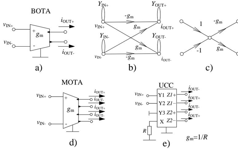
**Figure 5.2** a) schematic symbol of the BOTA, b) modified M-C graph of the BOTA, c) simplified M-C graph of the BOTA, d) schematic symbol of the MOTA, e) possible implementation of the MOTA using the UCC
