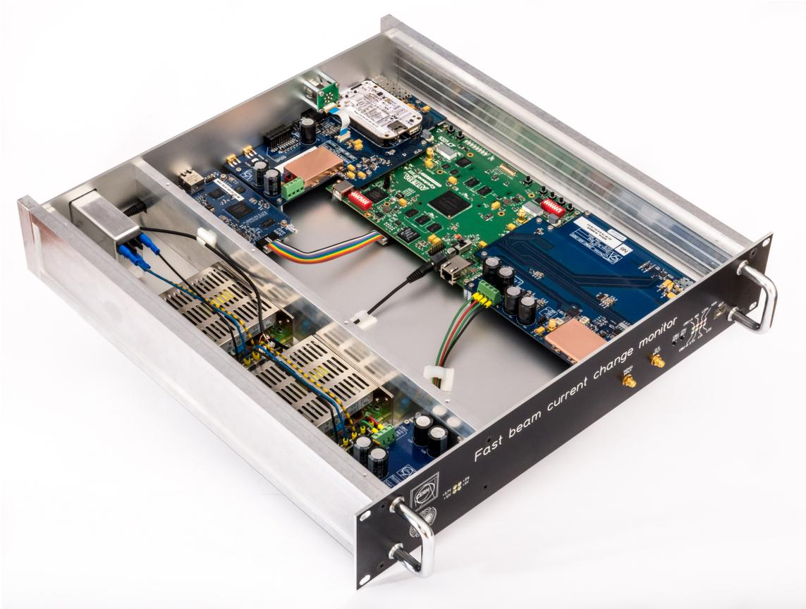
Fig. A.14: Perspective view of the FBCCM device without top panel
