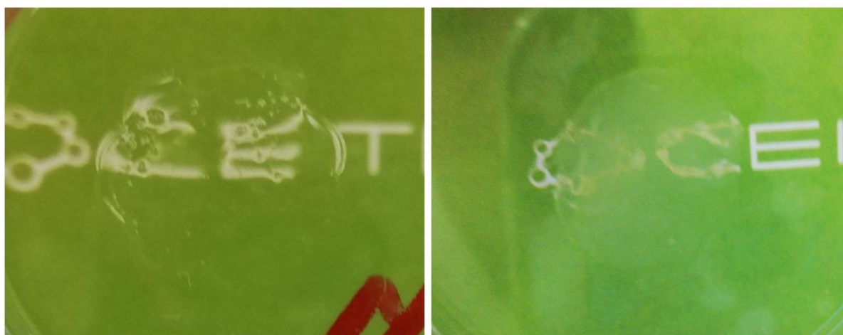
Figure 22: Comparison of hydrogel without (left) and with crosslinker PEGDA (right).
