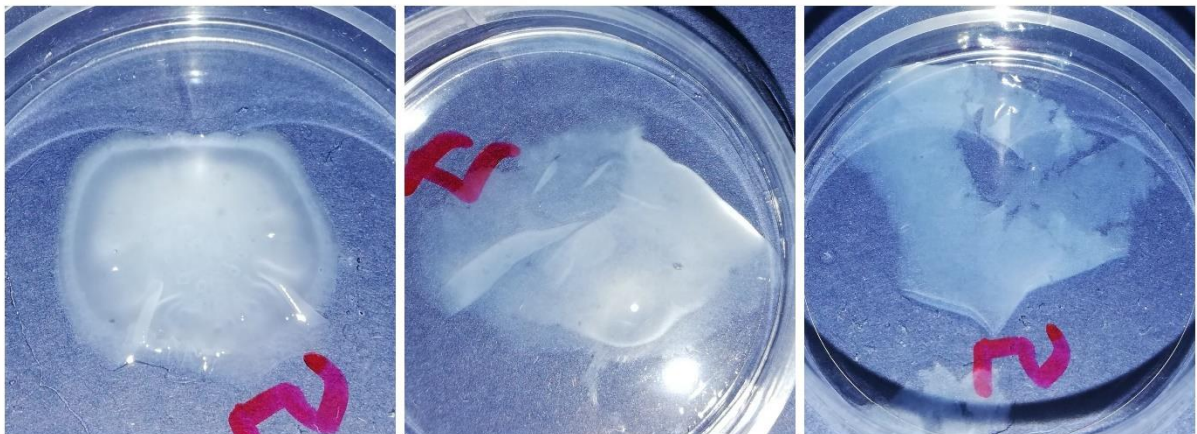
Figure 29: Swelling of hydrogels formed with crosslinker PEGDA. Before water uptake (left), after 1 day (middle) and 6 days (right).
