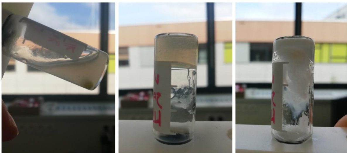
Figure 14: Visual representation of the phase transitions. The photo on the left shows a sol, the middle one a gel (at 37 °C) and the right one a suspension.
