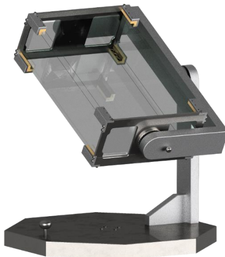
Figure 34 3D MGSE with mounting options [39]
